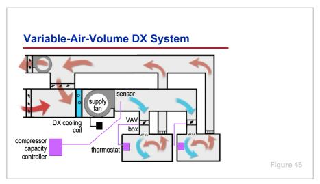
As mentioned previously, a VAV system varies the quantity of air supplied to the space in order to satisfy the load. The supply temperature is held constant in this system.
